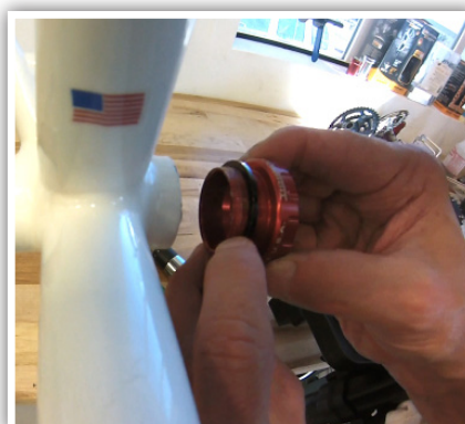
6. Insert non-drive side cup into frame, add supplied spacers as necessary to achieve proper bottom bracket width.
