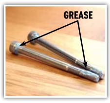
4. Apply a thin layer of grease to the bolts on both the threads and beneath the head.
