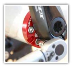
10. Using torque wrench, tighten both M6 x 75 to 8-10 Nm.
