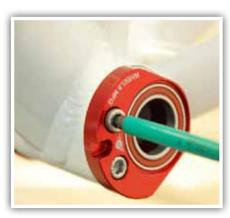
5. Thread in both M6 x 75 bolts, but do not fully tighten. Position the cups so that the bearings are facing towards the rear of the bike.
