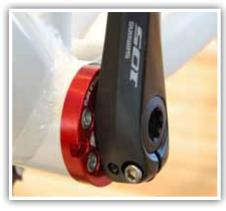
8. Tighten crank to manufacturer specifications.
