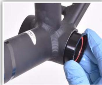
8. Insert non-drive side (male) cup by hand. Check that any internal wires or hoses are out of the way of the cup.
