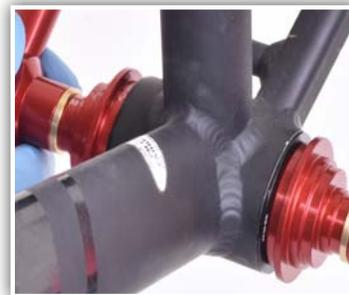
9. Using Wheels Mfg Universal Bottom Bracket Press [PRESS-7 or PRESS-7-PRO], insert one BB adapter into each bearing. Match the correct size step on the drift with bearing inner diameter. Slide press handle + rod thru BB adapters and cups.
