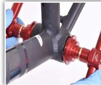
10. Spin on second press handle and fully tighten until non-drive side cup is flush with frame.
