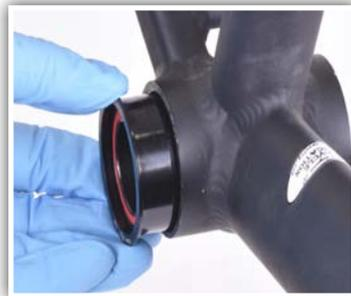
3. Insert drive side cup (female) into frame by hand. Check that any internal wires or hoses are out of the way of the cup.
