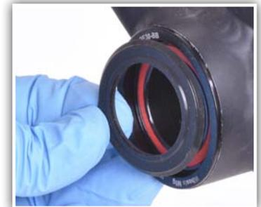
11. Outer silicone dust seals are placed directly against bearings. For added sealing, apply grease between seal and bearing.
