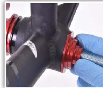
5. Slide second BB adapter onto threaded rod and into the opposite side of the bottom bracket shell. Match the correct step size with the BB shell inside diameter. Adapter should fit with little to no play.
