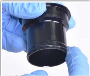
7. Apply a thin layer of grease to the inner o-ring on the male cup.
