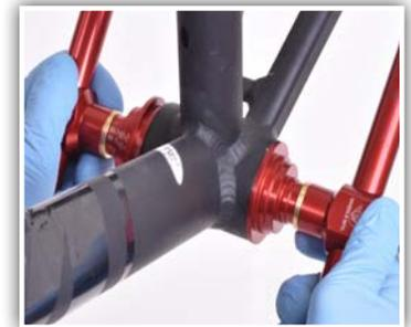
6. Spin on second press handle and fully tighten until drive side cup is flush with frame.
