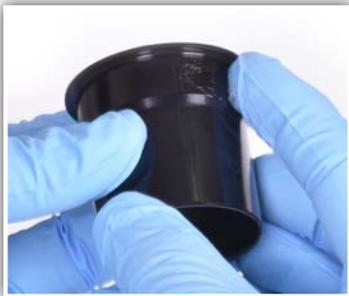
2. Apply a thin layer of high quality, carbon-safe grease or anti-seize compound to outside surface of each BB cup.
