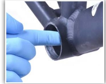
1. Thoroughly clean frame's bottom bracket shell. Do not install cups dry. Apply a thin layer of high quality, carbon-safe grease or anti-seize compound to inside surface of the shell.
