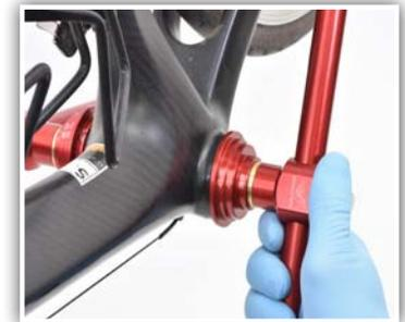
7. Spin on second press handle and fully tighten until drive side cup is flush with frame.
