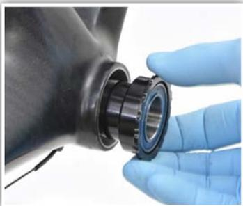
8. Insert non-drive side cup (male threads) by hand and turn clockwise until threads begin to engage. Do not cross-thread cups. Check that any internal wires or hoses are out of the way of the cup.
