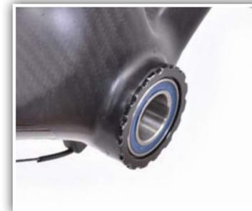
11. Bottom bracket is now installed. Install crankset per crank manufacturer's instructions.
