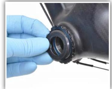
12. Outer silicone dust seals are placed directly against bearings. For added sealing, apply grease between seal and bearing.
