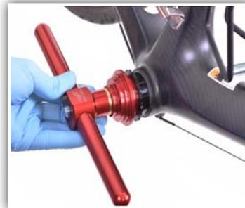
5. Using Wheels Mfg Universal Bottom Bracket Press [PRESS-7 or PRESS-7-PRO], insert one BB adapter into drive side bearing. Match the correct size step on the drift with bearing inner diameter. Slide press handle + rod thru BB adapter and cup.
