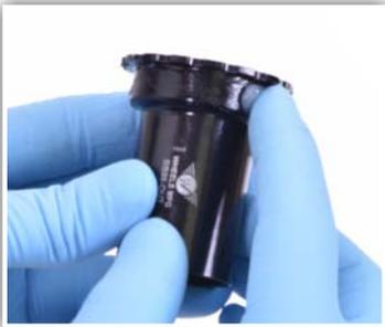
3. Apply a thin layer of high quality, carbon-safe grease or anti-seize compound to outside surface of each BB cup.
