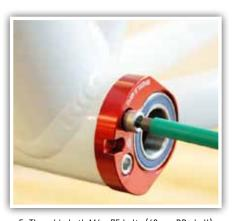
5. Thread in both M6 x 75 bolts (68mm BB shell) or M6 x 80 bolts (73mm BB shell), but do not fully tighten. Position the cups so that the bearings are facing towards the rear of the bike.
