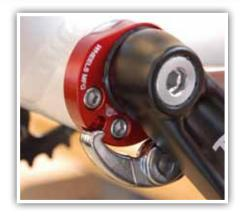
With rear wheel and chain installed, use spanner wrench (<u>TOOL-SPAN</u>) to rotate the EBB counter-clockwise until proper chain tension is reached.
