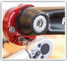
10. Using torque wrench, tighten both M6 x 75 (68mm BB shell) or M6 x 80 (73mm BB shell) holts to 8-10 Nm
