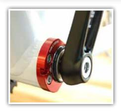
Install left crank arm, making sure outer dust seal is installed. Use crank spacers as needed to take up any play. Remove spacers as necessary if binding occurs.
